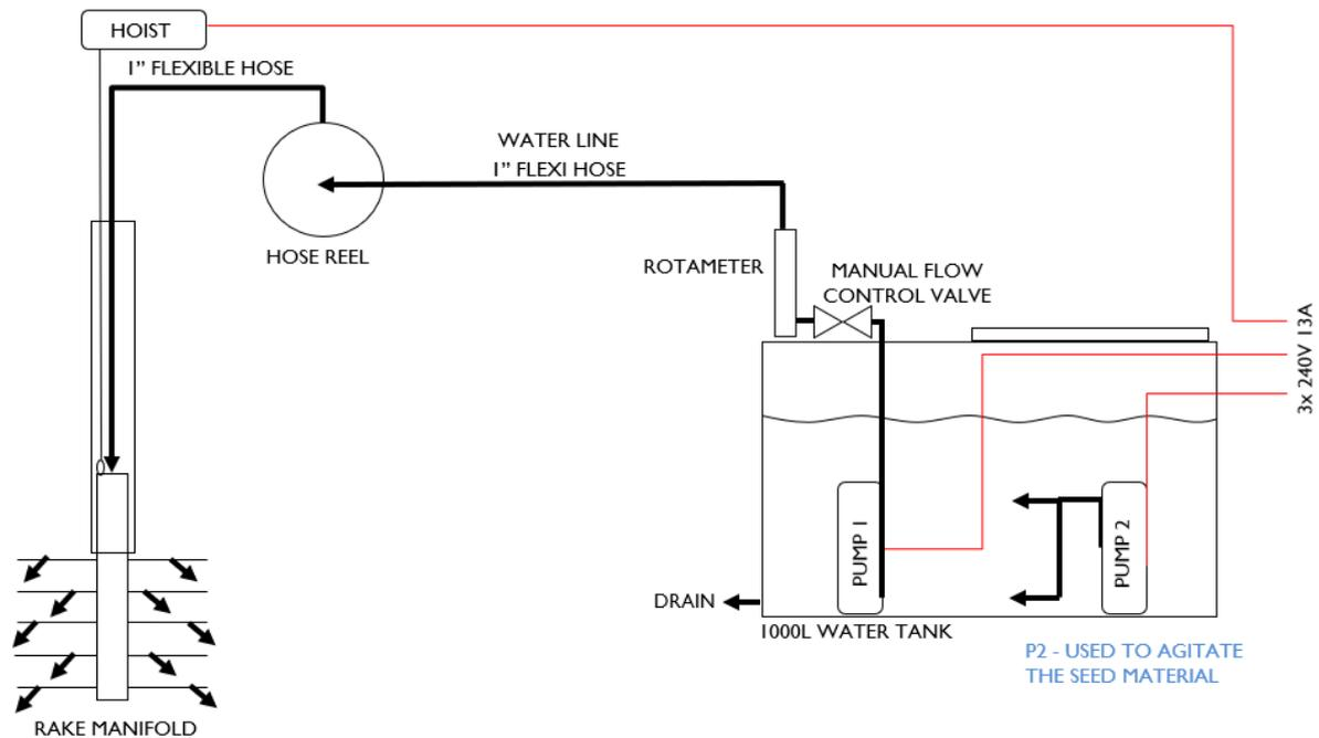
The basic components of the SCITEK Tow Tank seeder are shown in the schematic diagram shown above. It comprises of the rake which is essentially five rows of metal tubes with multiple holes drilled on the wall of each tube that are used to discharge water that is premixed with hollow glass spheres. The rake is designed to spread the seeding evenly in the area of interest.
