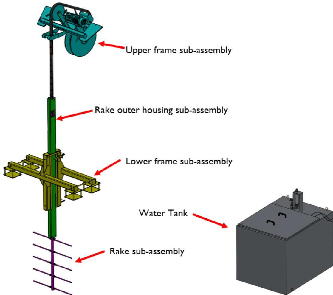
The SCITEK Tow Tank seeder with all its sub-assemblies is shown above and these are explained in more detail below.
