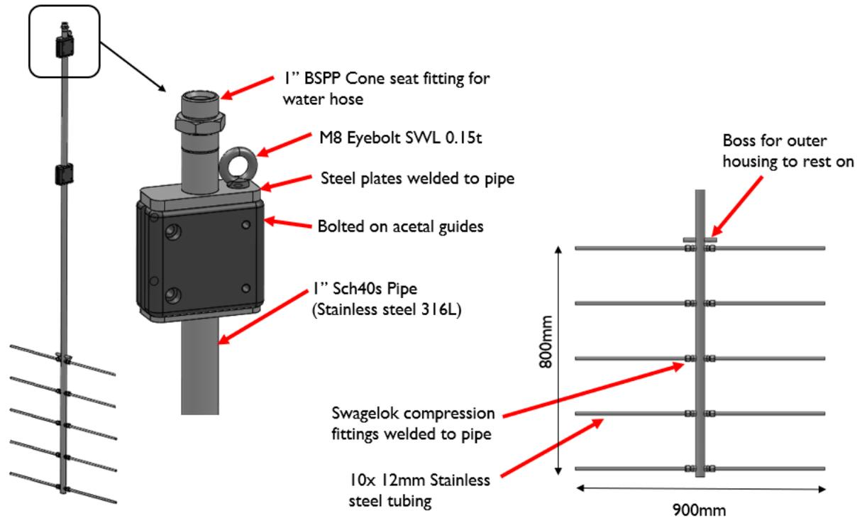
The rake assembly can also be custom made to suit customer requirements. The retractable boom can immerse the rake up to a depth of 2.5meters.
