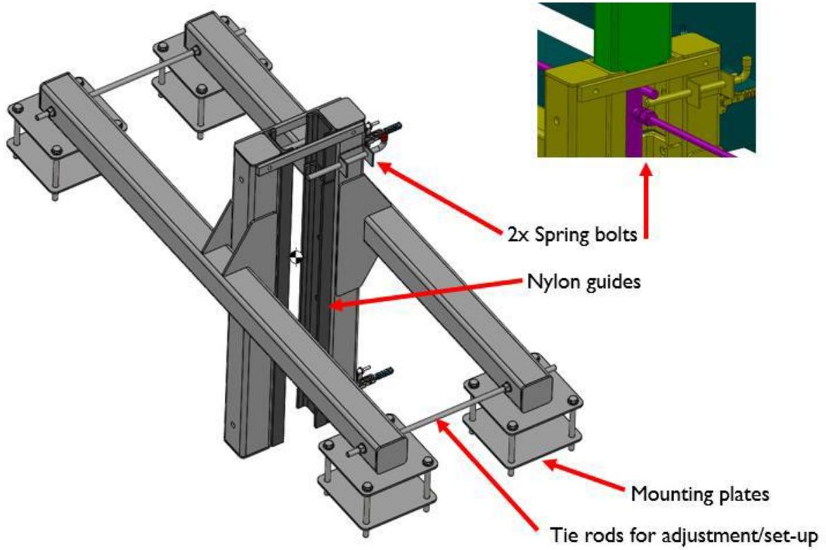
This assembly is normally custom made by SCITEK to suit installation on the customer's carriage.
